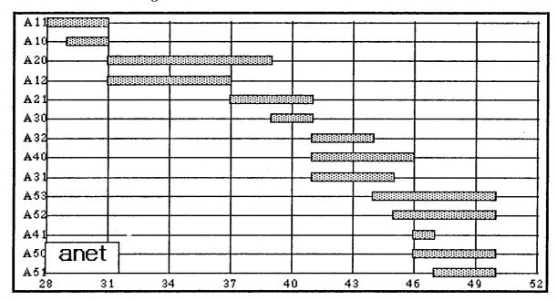
This View shows the activities along the vertical axis and time along the horizontal axis. In this particular view, only one time schedule for each activity is shown. Through varying the shading, it is quite easy to extend the presentation to include how much each activity may *float* in time without upsetting the overall project schedule.
