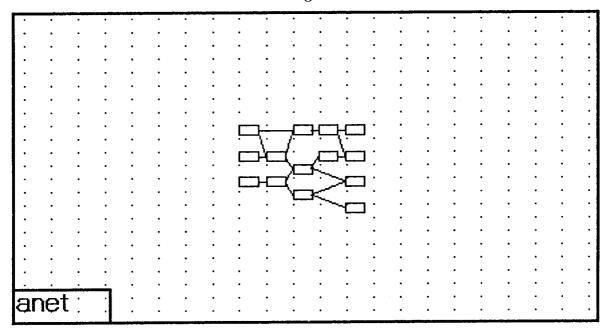
This View provides an alternative to the previous example. The symbols are smaller, and it therefore possible to present a larger part of the network on the screen. The small symbol size makes it impractical to print the activity name in the symbol, and the user must get this information by some other means.
